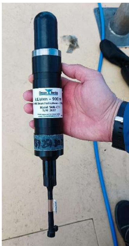
Figure 3.5. Hydrophone for acoustic measurements of noise radiated by the gas bubble oscillating walls.
