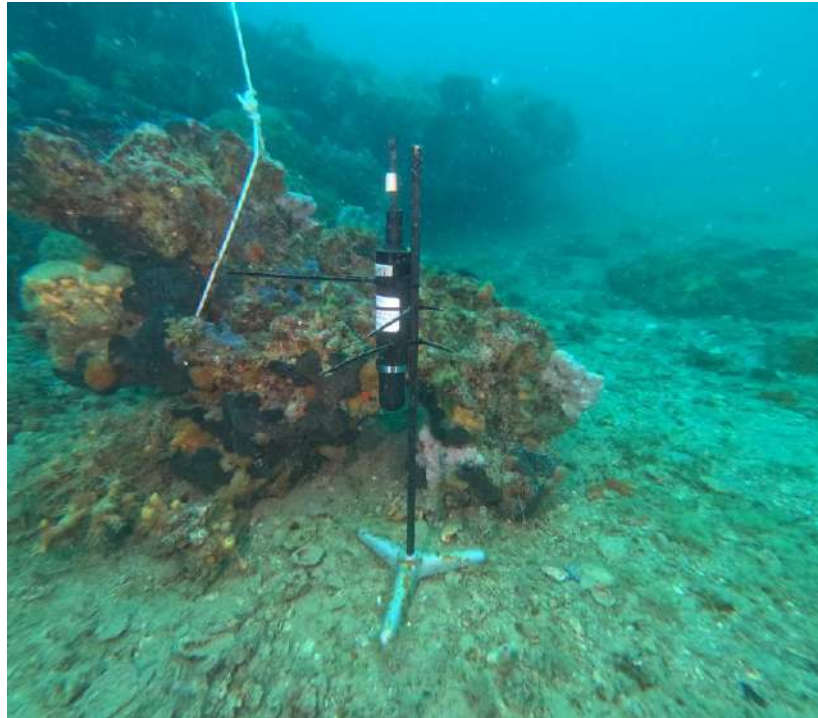
Figure 4.20. Hydrophone recording the noise radiated by the gas bubble oscillating walls in the “San Pietro” station.
