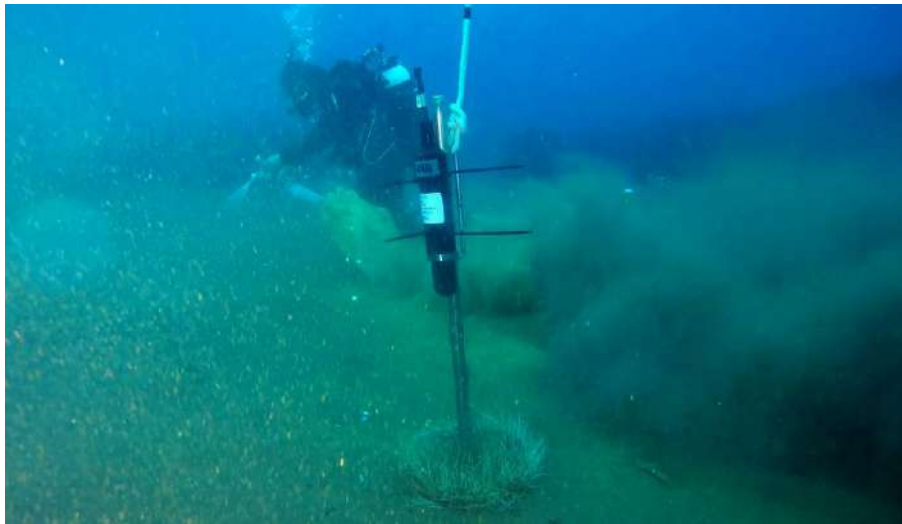
Figure 4.5. The INGV hydrophone deployed in one of the hot patch detected in “Hot/Cold1”, in the proximity of a not-stationary bubble seep. Diver pursuing sampling activities in the background.
