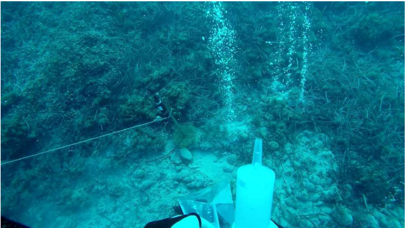
Figure 4.4. Hydrophone recording the noise radiated by the gas bubble oscillating walls in the “Black Point Bubbling” site.
