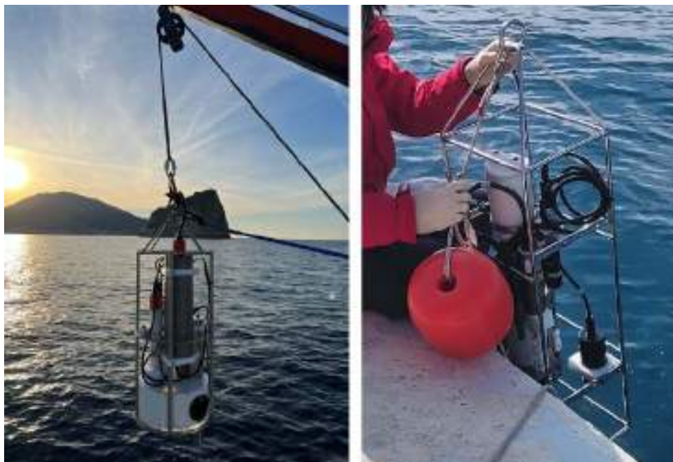
Figure 3.2 Multiparametric probes employed during the project field activities. On the left: RBRmaestro equipped with a multichannel logger and CONTROS Hydroc CO 2 and CONTROS Hydroc CH 4 sensors. On the right: SBE19plus V” equipped with pH, fluorometer/turbidimeter and dissolved oxygen sensors.
