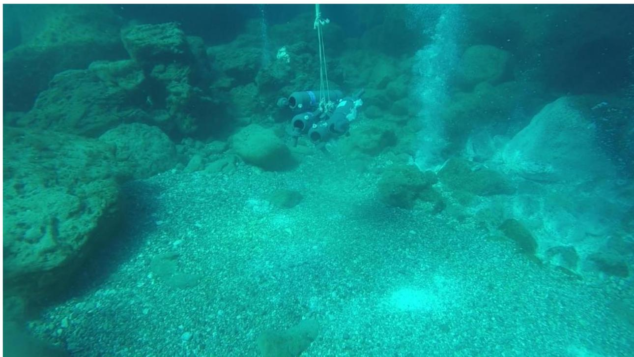
Figure 4.9. Deployment of Niskin bottles in “Bottaro Single”.
