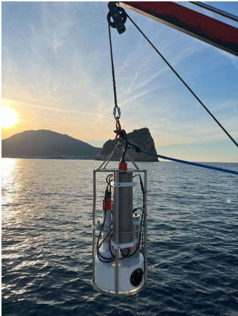
Figure 3.3. Multi-parametric probe deployment in “Black Point Bubbling”.
