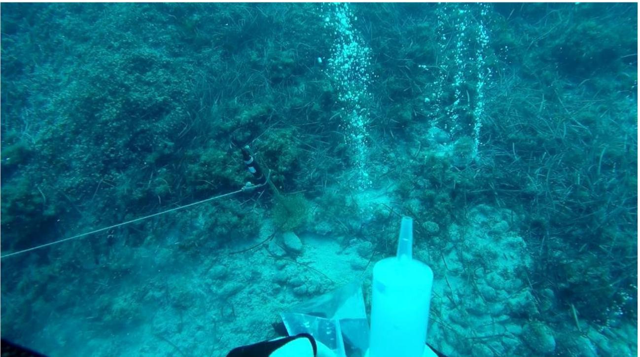
Figure 4.2. Hydrophone recording the noise radiated by the gas bubble oscillating walls in “Black Point Bubbling” station.
