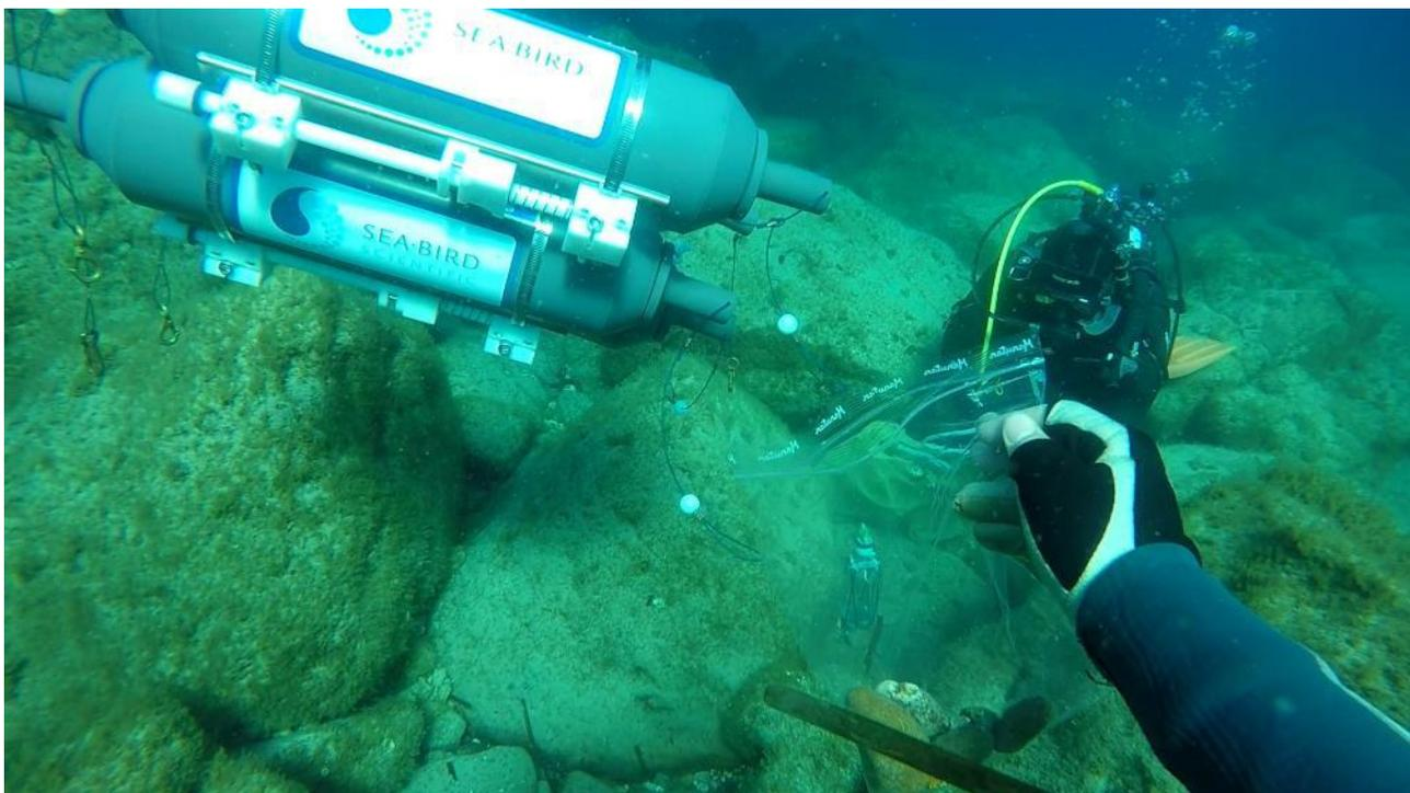
Figure 4.11. Niskin closure and sediment retrieval from “Bottaro Downstream” rocky seabed.
